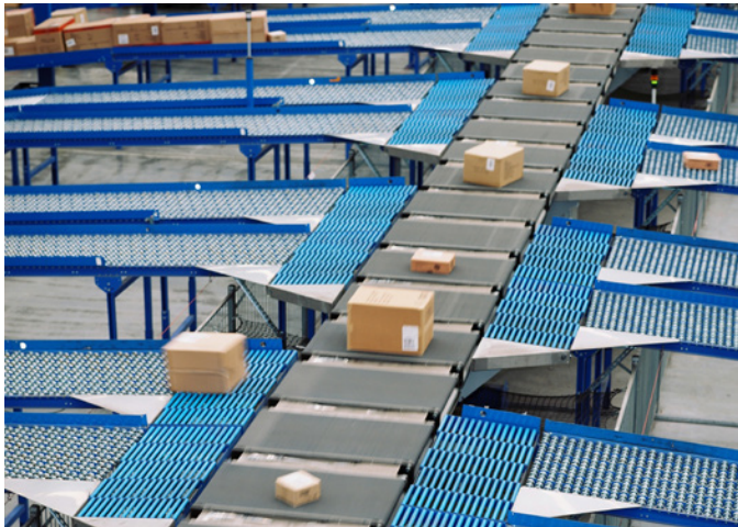
The Crossbelt Sorter handles a broad range of items including plastic totes, cardboard cartons, trays, stuffed envelopes, and poly bags.
