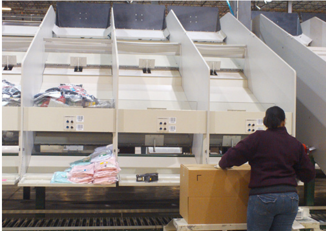
The Crossbelt Sorter is configured as an order consolidator. Apparel items are sorted to a packing chute.
