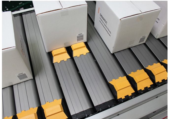
The Sliding Shoe Sorter with parallel divert maximizes throughput rates.
