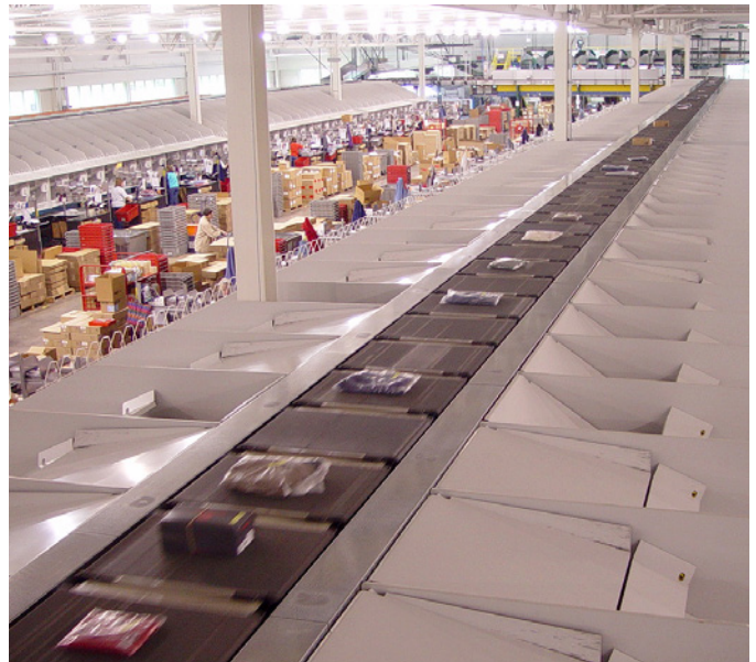
The Crossbelt Sorter diverts to packing chutes on two sides.
