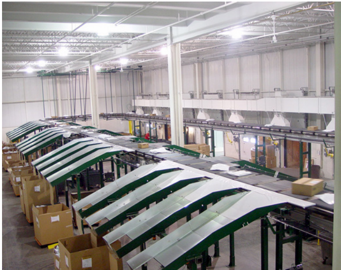
The Crossbelt Sorter functions as a shipping sorter.
