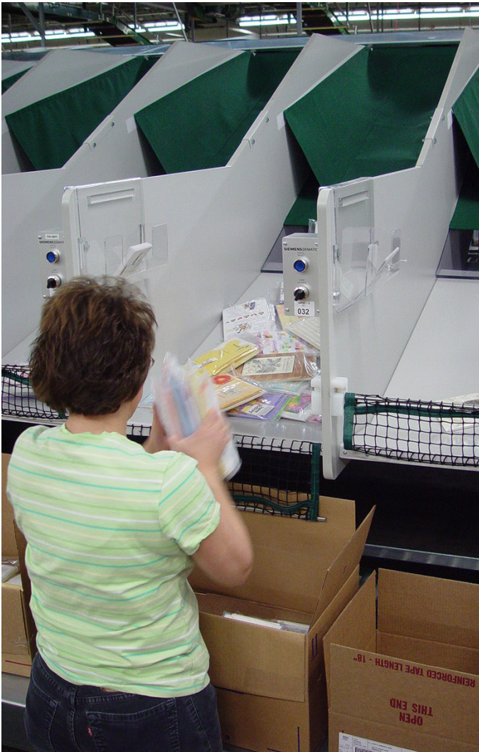
General merchandise is sorted into a packing chute at a retail store replenishment center.
