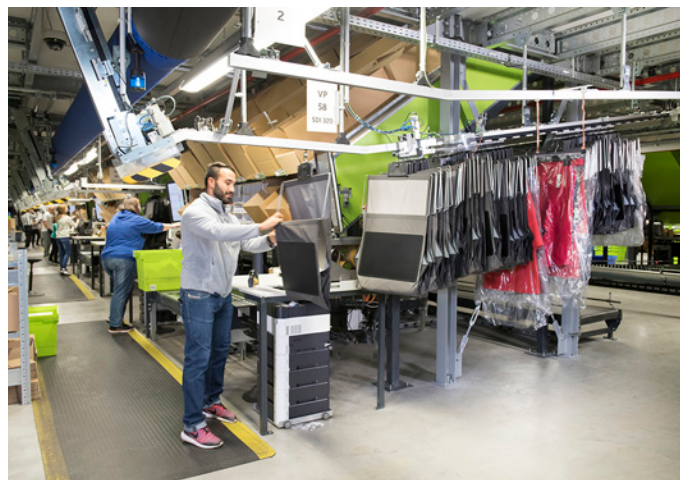
All the items for a customer order arrive at the packing workstation in a precise sequence.
