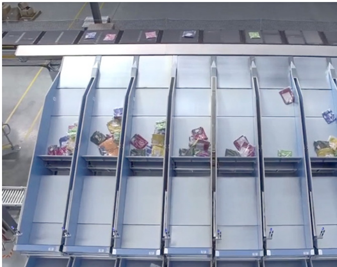
Apparel items in poly bags are sorted by a Crossbelt Sorter to chutes and then packed.
