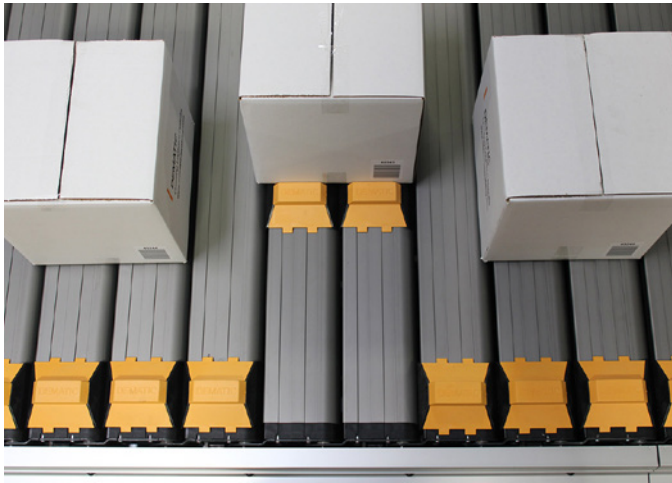
The Sliding Shoe Sorter provides parallel diverting with minimal gaps between cartons to support higher sorting rates.
