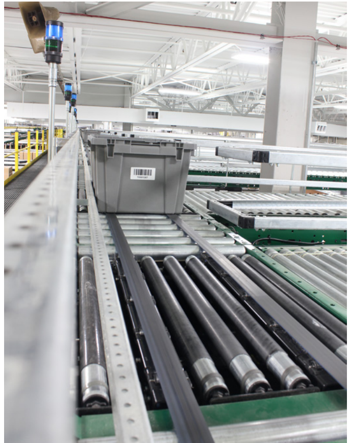
The two belt configuration accommodates totes.
