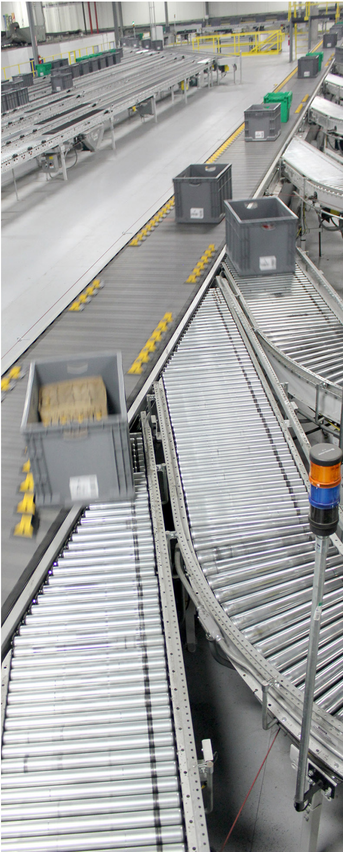
The Sliding Shoe Sorter is available with angle divert.
