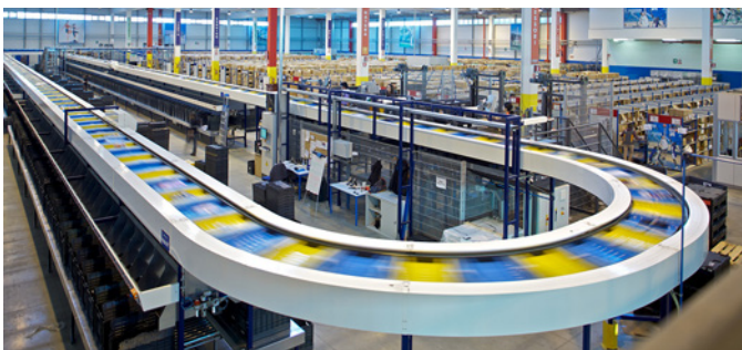
The Split-Tray Sorter is an ideal solution for order consolidation applications.
