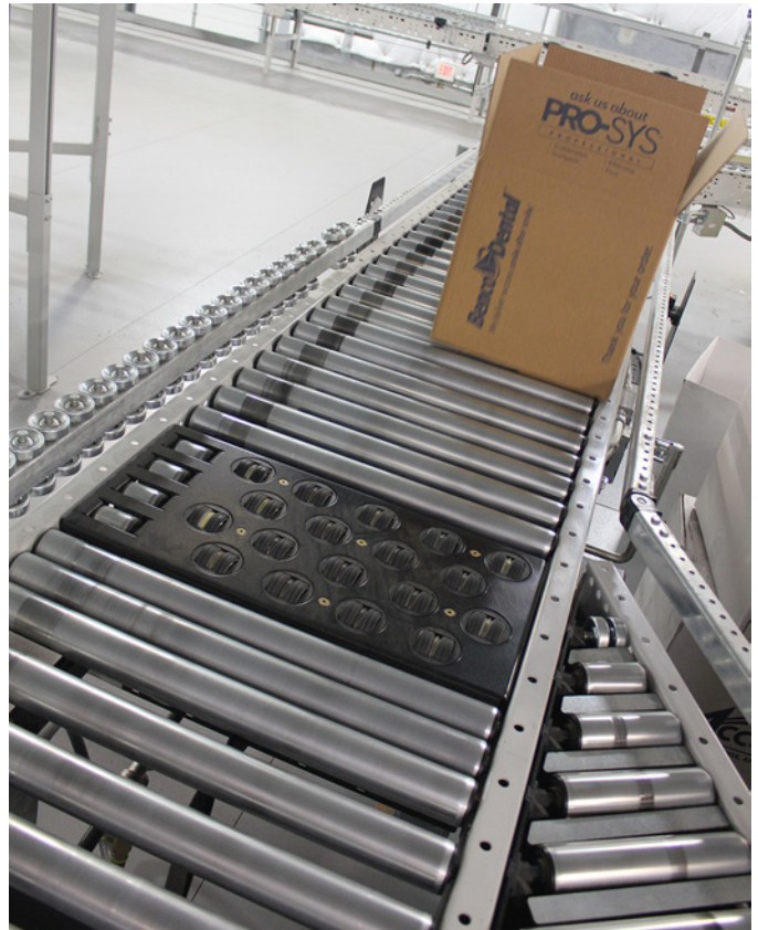
The Steerable Wheel Sorter diverts order cartons to packing workstation.
