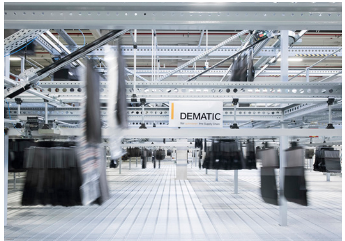
Each pouch is sorted and held in a dynamic buffer until released by the WES.
