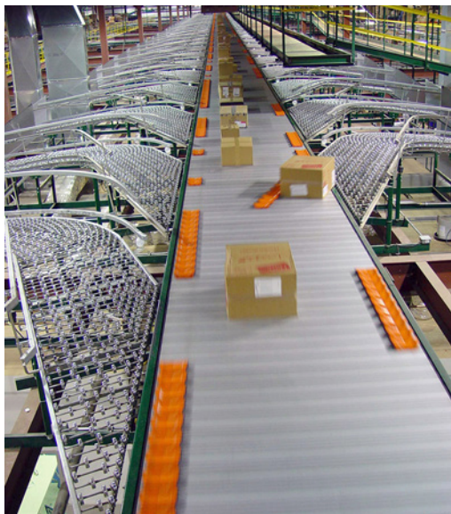
The two-sided sorter is ideal for cross-docking applications.
