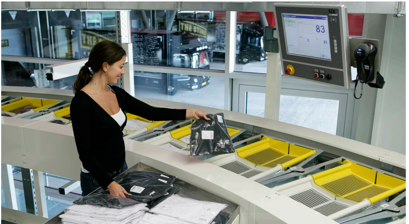
The Split-Tray Sorter enables high rate sorting of single items.
