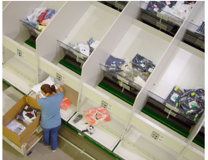
The Crossbelt Sorter diverts apparel in poly bags to order consolidation chutes.
