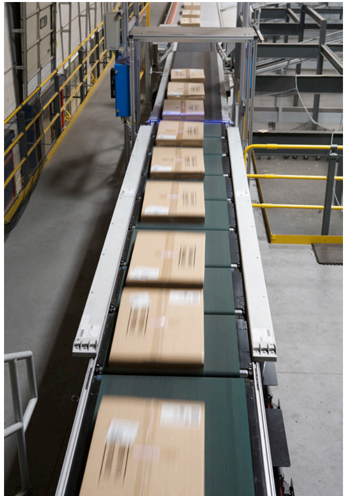
Induction to the Sliding Shoe Sorter is optimized with the eight belt carton gapping conveyor.
