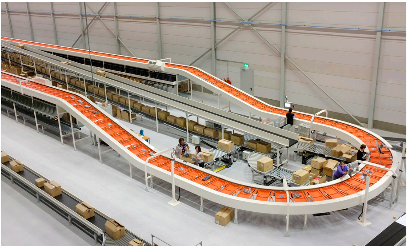
The Split-Tray Sorter implemented with workstations at floor level.
