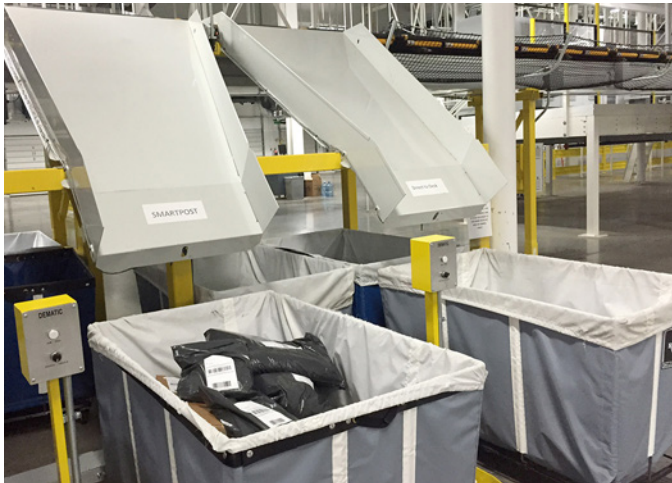
The Crossbelt Sorter diverts bags into a parcel shipping container at an e-com fulfillment center.
