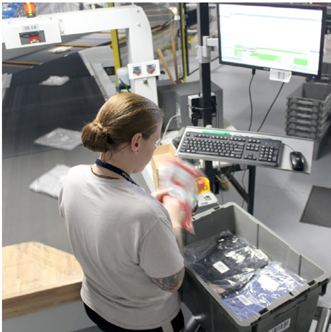
Batch picked items are manually inducted onto the Crossbelt Sorter.
