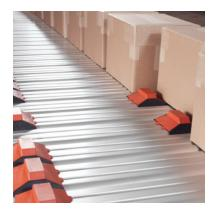
FlexSort overcomes this problem by utilizing an independent premium-efficiency drive for each belt in its FlexGap<sup>™</sup> gapping device, equipped with a high-performance, variable-frequency controller instead of a servo-controller. The motor is driving each zone (belt) independently, so there is no gear reduction, giving very good control over the ratio from the speed of one belt to the next. This means more precise gapping.
